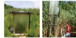
Figure 5.6 Chamber volume must be adjusted to enclose plants of different stature (A & C). (B). © Rachel Hagar, SERC; C. Eric Heatherton, SERC
